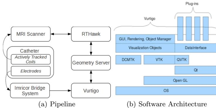
**Fig. 1.** Design. a) Communication pipeline. Vurtigo is able to passively receive information from the MRI scanner or actively prescribe the scan. EP catheter recordings are via the Imricor bridge system. b) Software components and libraries.
